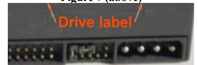
Two-jumper Maxtor Set as "Master"
