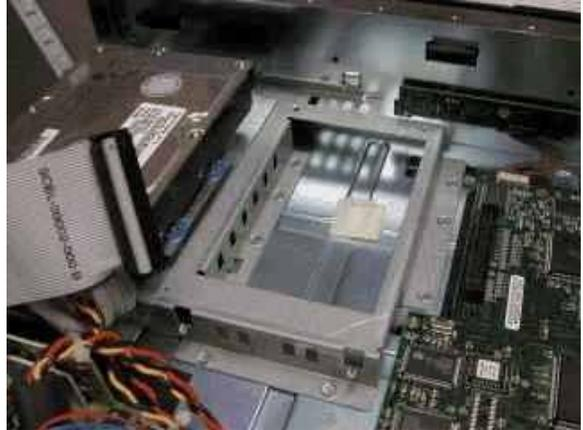
**STEP 7:** Slide the drive bracket into position, lining up the two metal prongs in the TiVo chassis with the holes in the TiVo Mounting Bracket. If you find that the factory-installed bracket is too close to the new bracket that you are now trying to install, you may have to unscrew the factory bracket (which is connected to the factory drive) and move it into the alternate set of holes. Moving the factory bracket over will leave sufficient room for the new bracket.
