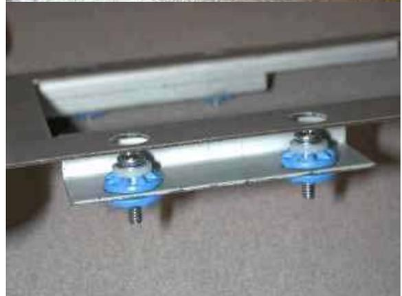
**STEP 4:** Turn the disk drive so that the screw holes in the disk drive line up with the screws in the bracket. Using a Phillips screwdriver, tighten all 4 screws. Note that the connectors are sticking out at the left side of the disk drive.
